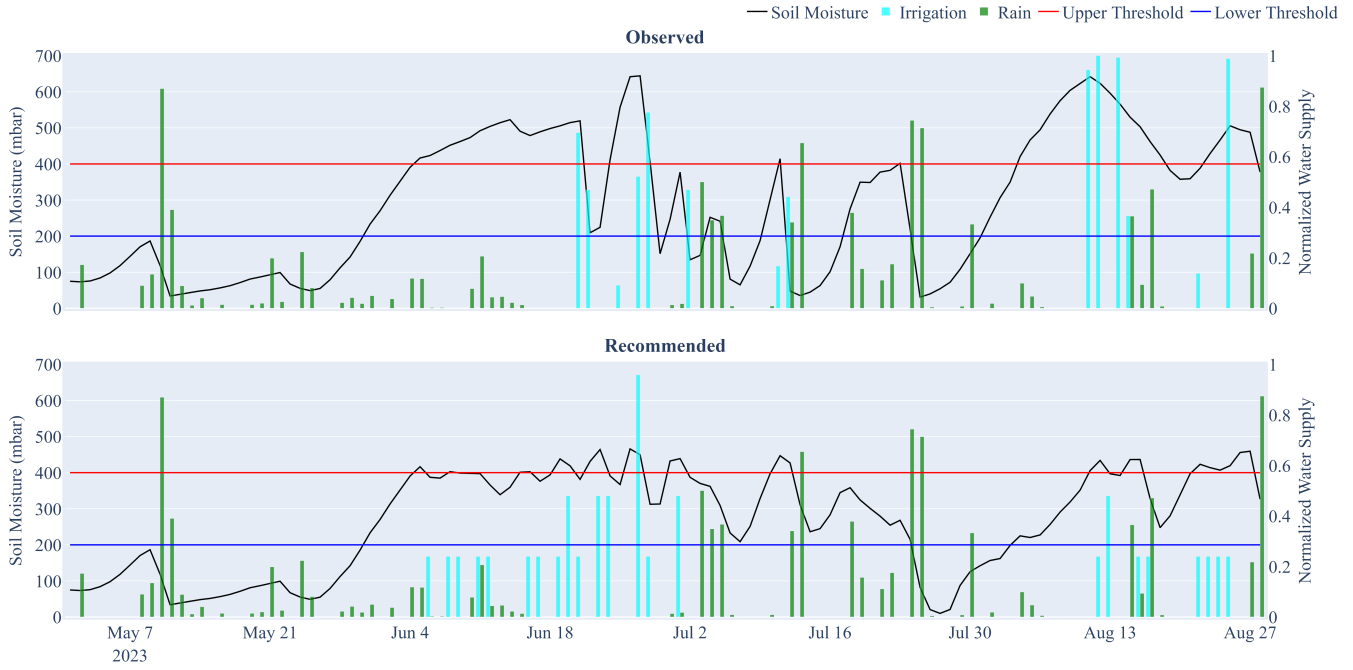
Fig. 2. Comparison of actual and DSS-simulated irrigation schedules for a specific water sector in RDL during 2023. The upper graph shows the real tensiometer readings and irrigation events, while the lower graph displays the simulated trend based on DSS recommendations.
