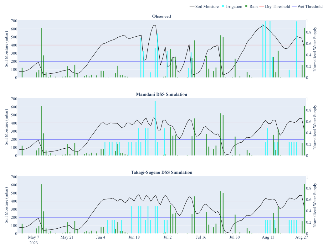
Figure 10. Comparison of actual and IDSS-simulated irrigation schedules for a specific water sector in the study area. The top subplot shows real tensiometer readings, rain, and irrigation events; the middle subplot presents simulations from the Mamdani-type IDSS; and the bottom subplot depicts simulations from the Takagi–Sugeno ANFIS IDSS. The red and blue horizontal lines represent the dry and wet thresholds defined by the agronomists.
